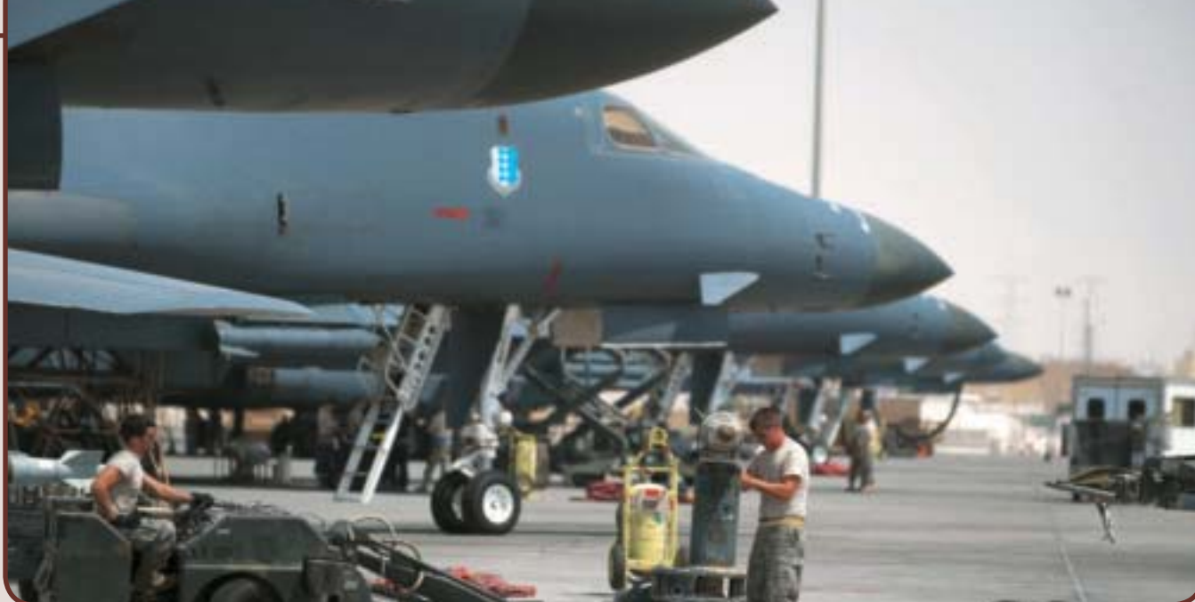
A1C Brian Adkins secures a GBU-38 Joint Direct Attack Munition to an MJ-40 bomb lift truck operated by SrA. Adam Weaver in Southwest Asia in 2009. The JDAM is then loaded onto a B-1B for a sortie.
